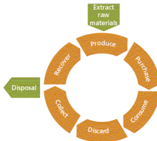
Figure 2 The circular (or 'closed loop') approach to waste management (Defra, 2007)
